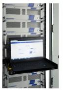
Appearance: Option drawer with control PC mounted in 19" system rack.
